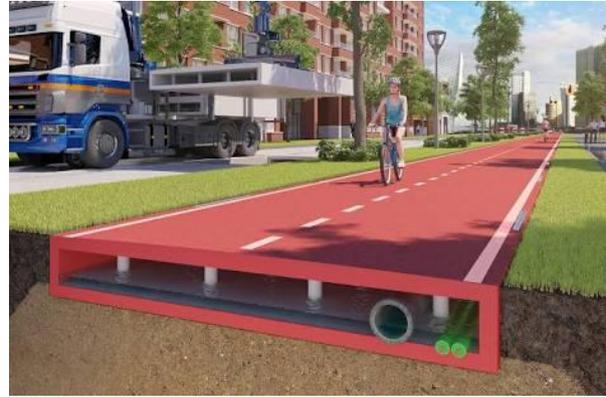
preventing excavation damages. The PlasticRoad is a completely circular product that is made from recycled plastic. PlasticRoad is simple, efficient, low cost and easier to construct. It is sustainable, light weight, easy to repair and has prolonged life expectancy than normal road. **The PlasticRoad can be constructed using plastics from Deonar Dumping ground.**
