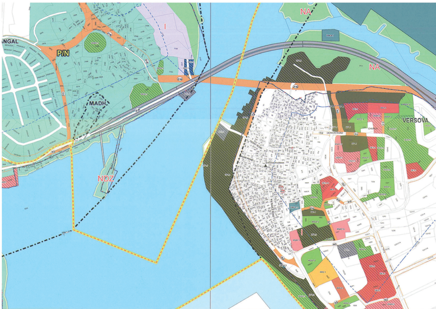
PROPOSED DEVELOPMENT PLAN FOR 2034 IT PROPOSES WIDENING OF THE PATIL GALLI(18.3) FROM 6M TO A 18M WIDE ROAD. THIS ROAD WOULD JOIN THE PROPOSED COASTAL ROAD (27.45) AND IN TURN MAKE IT A TRAFFICATED ONE.
