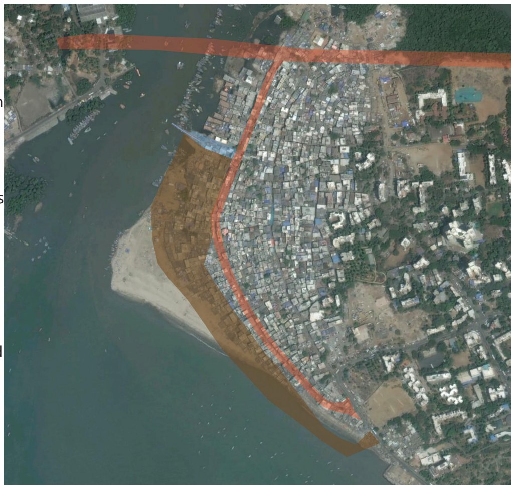
PROPOSED DEVELOPMENT PLAN FOR 2034 IT PROPOSES WIDENING OF THE PATIL GALLI(18.3) FROM 6M TO A 18M WIDE ROAD. THIS ROAD WOULD JOIN THE PROPOSED COASTAL ROAD (27.45) AND IN TURN MAKE IT A TRAFFICATED ONE.
