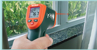
Checking for heat loss around windows and doors
