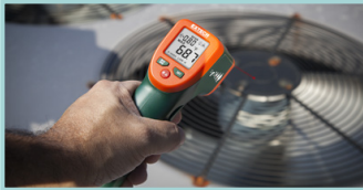
Test for temperature in HVAC systems
