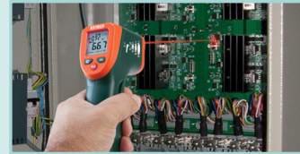
Detect hot spots on circuit breaker panels
